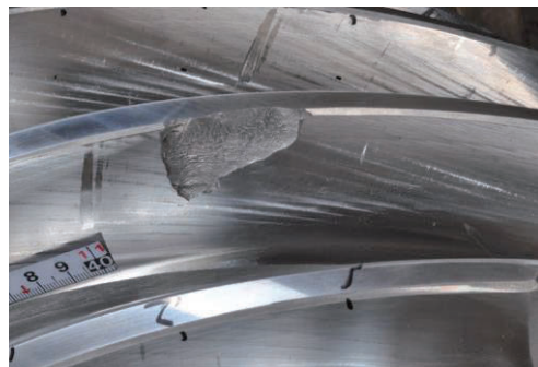
Fig.1 Tooth flank damage experienced
